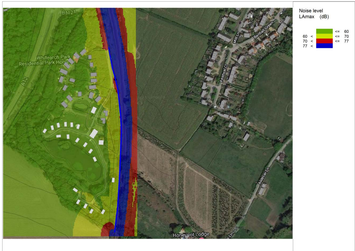
Plate 3.1: Noise contours for Whitearch Park – with acoustic barrier adjacent to railway line
